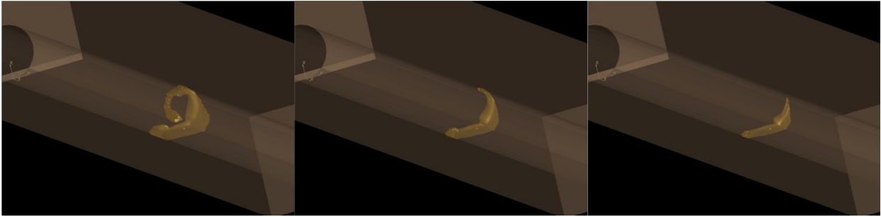
Figure 3. Predicted 4 % v/v H 2 iso-surface at 1, 6, 10, 20, 30 and 40 sec for the car scenario.
