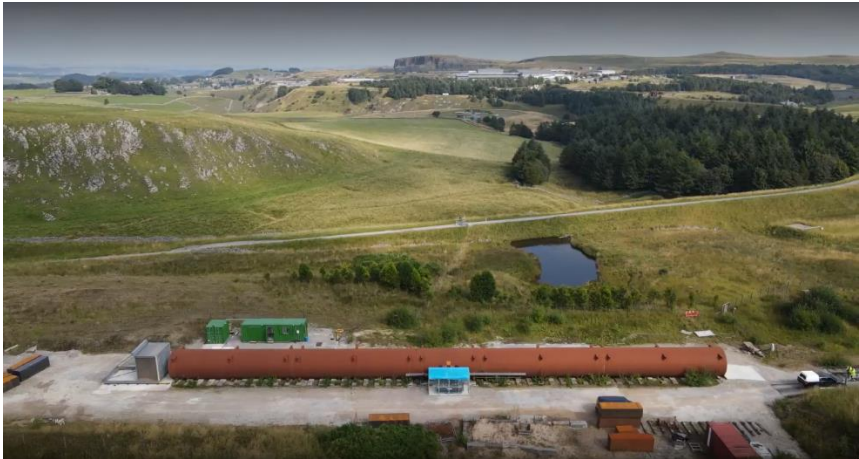
Figure 1: Image of the tunnel, gas delivery rig (centre) and fan structure (left).
