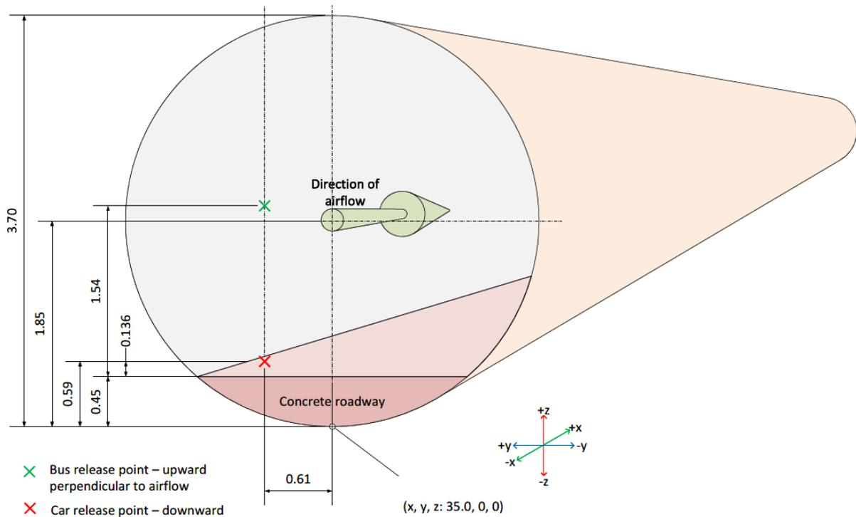
Figure 5: Cross-section sketch of the release point of the tunnel (section through the mid-point of the tunnel at  $x=35.0$  m)
