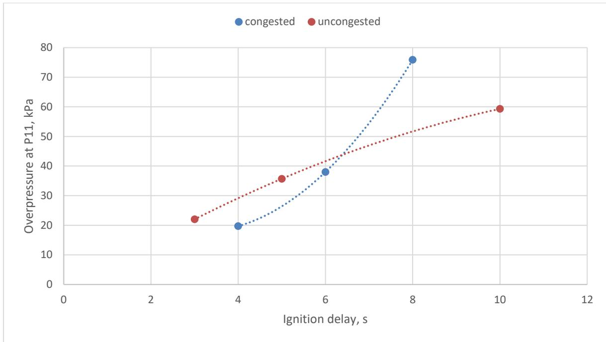
Figure 8. Comparison of the generated overpressure for releases of hydrogen at different ignition delay times and with and without congestion.
