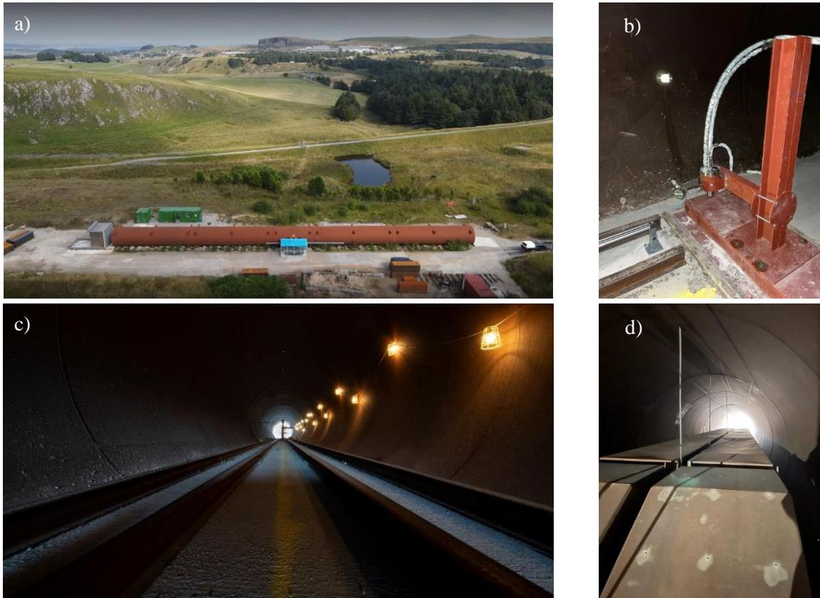
Figure 1. a) Aerial image of 70 m steel tunnel, b) discharge nozzle manifold, pointing downward, c) Inside the 3.7 m diameter tunnel showing the tracks used to secure scaled vehicles, d) scaled trains secured to tracks with thermocouple arrays also visible.
