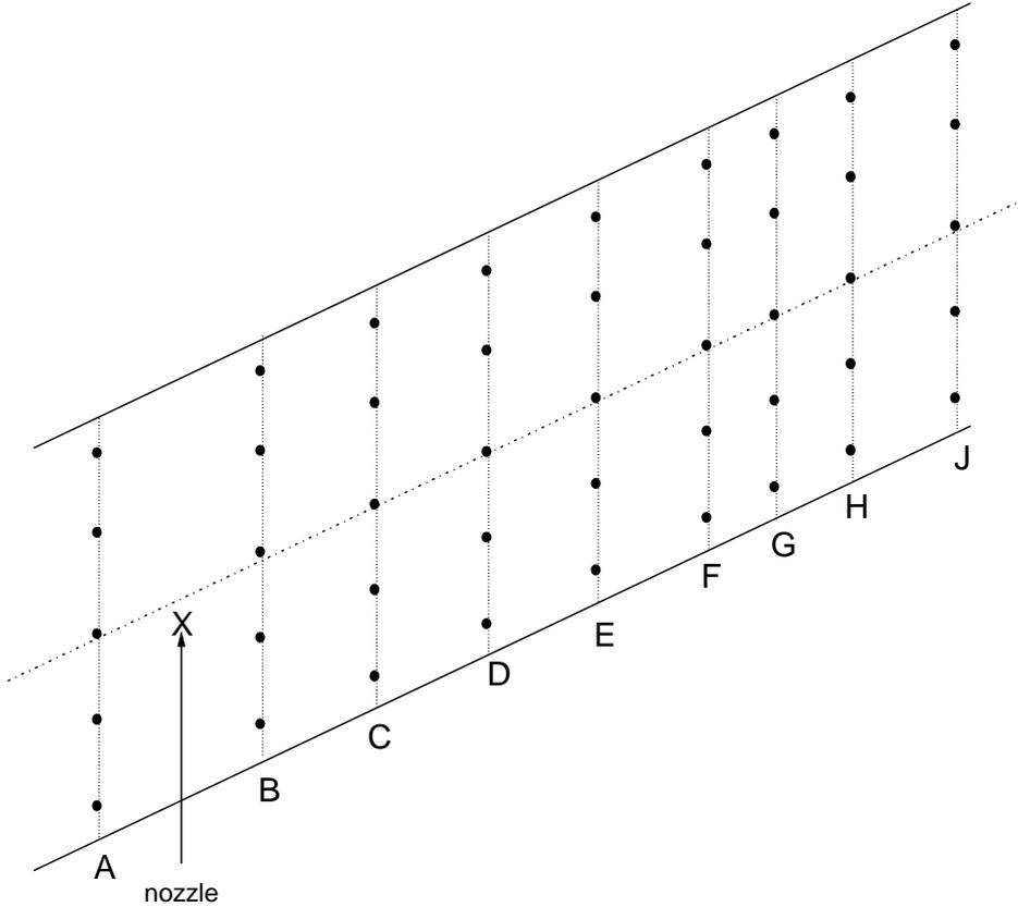
Figure 6. 3-D representation of thermocouple flame sensor locations relative to release point
