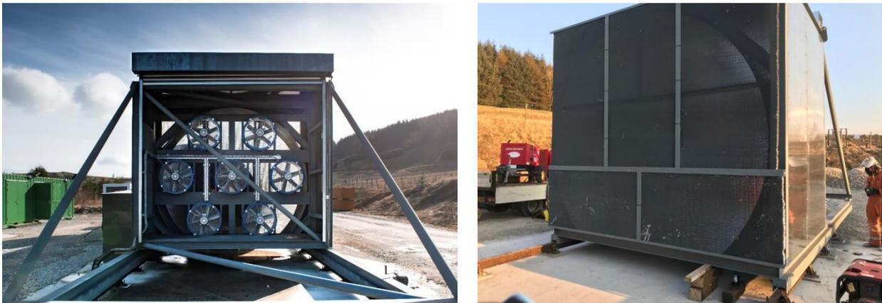
Figure 4. Fan array. Comprises 7 axial fans with a combined power output of 15.4 kW, capable of generating wind speeds up to 5 m/s inside the tunnel
