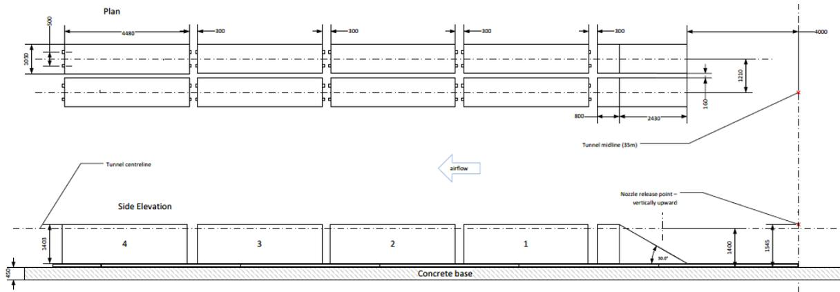
Figure 7. Layout and dimensions of scaled vehicles in HSE 70 m tunnel (distance from mid-line of tunnel ( $x = 35.0$ ) are indicated).
