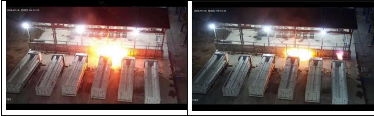
Figure 8 -A) Hydrogen leak from the hose in front of the trailer. No. 4 burst into flames; B) Hydrogen leaking from the loading and unloading ports on trailer No. 6 burst into flames (Source of the pictures: Investigation Report on the "7-30" General Leakage and Fire Accident at Dongguan Juzhengyuan Technology Company Limited, Lixia Island, Shatian Town, Dongguan City).
