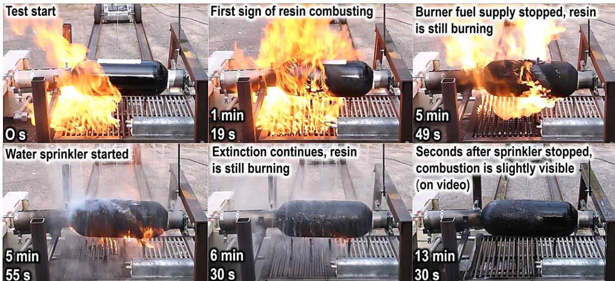
Figure 8. Snapshots of the \mu LNB tank prototype COPV#CB-5 behaviour in the fire test
