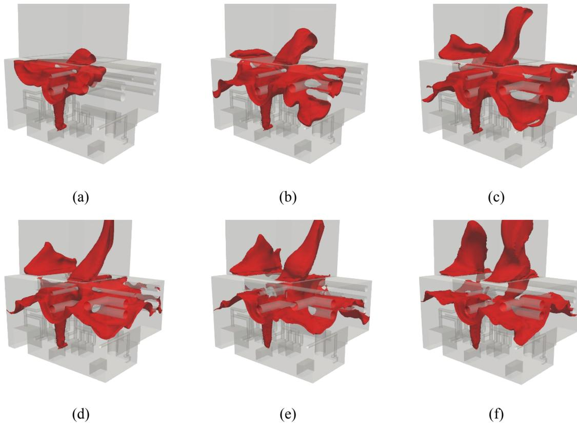
*Figure 3: Contour surface of hydrogen cloud at LFL concentration after (a) 3 s, (b) 6 s, (c) 9 s, (d) 12 s, (e) 15 s, and (f) 18 s from the leakage start.*
