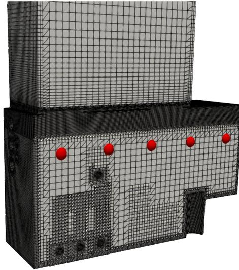
*Figure 2: Section in the computational grid with measuring points marked in red*
