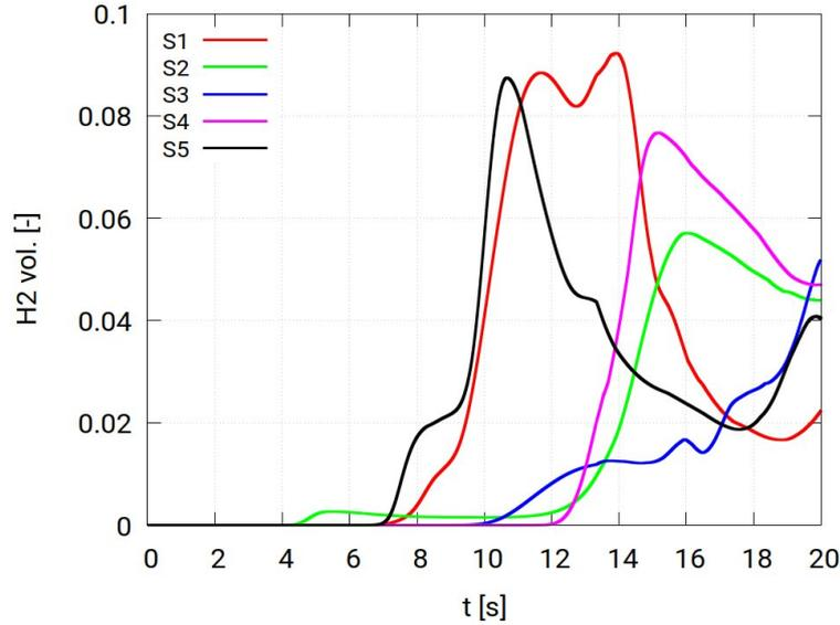
Figure 4: Hydrogen vol. concentrations development in the building at three different locations shown in Fig. 2.
