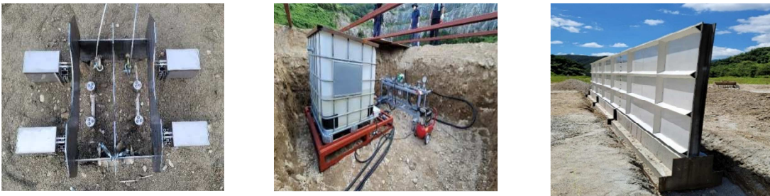
(a) Heptane nozzles and ignitor (b) Heptane fuel tank and supply system (c) Installed protective barrier
