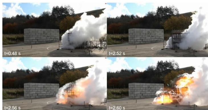
Figure 5. Stills images showing sudden gust immediately prior to ignition in Trial 23 [34].
