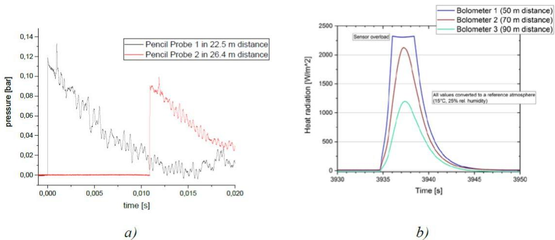
Figure 7. Overpressure and thermal radiation after the failure of an MLI-insulated vessel positioned horizontally filled with LH<sub>2</sub> (a) Blast waves measured at distances of 22.5 m and 26.4 m; (b) heat radiation from the burst of the MLI-insulated vessel [25,26].
