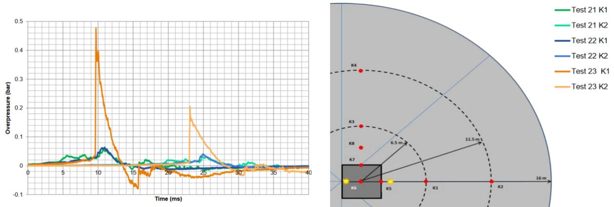
Figure 6. Overpressure comparison for the repeated trials 21 to 23 [34].
