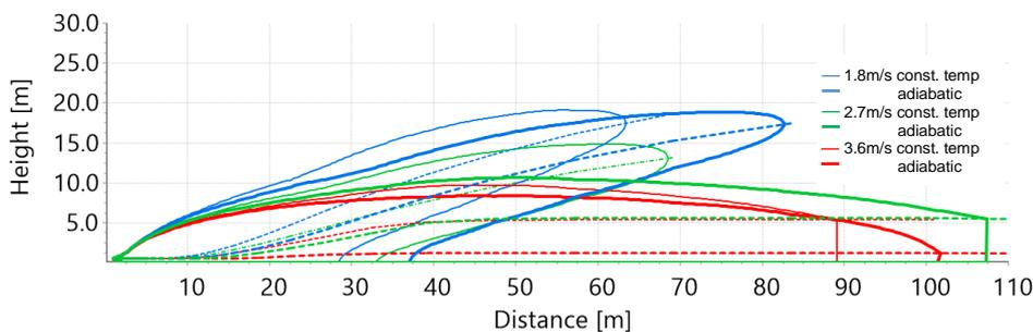
Figure 10: Simulations Test 6 with adiabatic and constant temperature boundary condition at the ground (surface roughness length 0.1m) for different wind speeds; comparison of cloud dispersion behaviour shown by trajectory and plume contour (2% concentration v/v)
