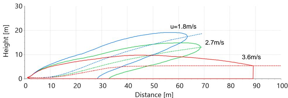
Figure 8: Simulations Test 6 (surface roughness length 0.1m) for different wind speeds; comparison of cloud dispersion behaviour shown by trajectory and plume contour (2% concentration v/v)
