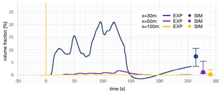
Figure 11: Comparison of maximum hydrogen concentrations during Test 6 (EXP) [6] compared with simulations from EFFECTS v12 (SIM)
