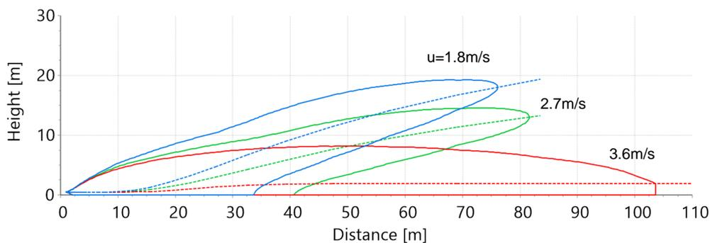
Figure 6: Simulations of Test 6 for different wind speeds; comparison of cloud dispersion behaviour shown by trajectory and plume contour (2% concentration v/v)
