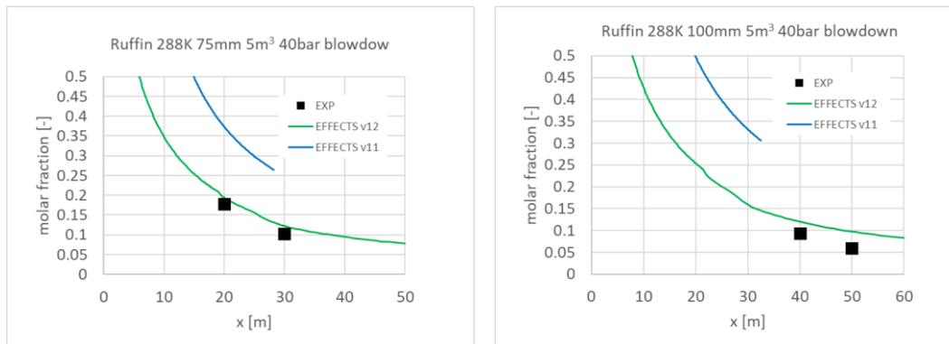
Figure 2: Hydrogen release experiment from a reservoir of  $5\text{m}^3$  (Ruffin), release at 298K, 40bar, 75mm hole, (left) and 288K, 40bar, 100mm hole (right); experimental data from [3], simulation with EFFECTS v12
