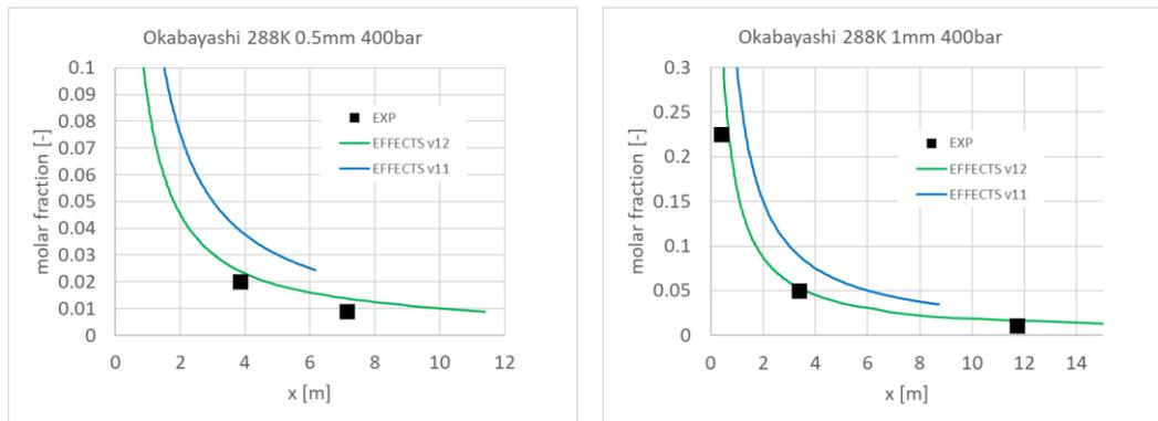
Figure 3: Hydrogen release experiment (Okabayashi) at 288K, 400bar, 0.5mm hole (left) and 288K, 400bar 1mm hole, (right); experimental data from [3], simulation with EFFECTS v12
