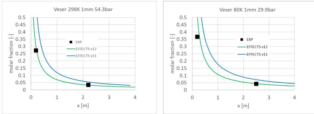
Figure 1: Hydrogen release experiment (Veser) at 298K, 54.3bar, 1mm hole (left) and 80K, 29.9bar, 1mm hole, (right); experimental data from [3], simulation with EFFECTS v12
