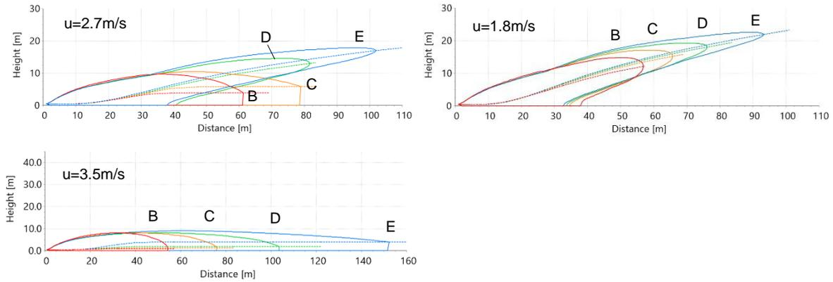
Figure 7: Simulations Test 6 for different atmospheric stabilities and wind speed of 2.7ms (a), 1.8m/s (b) and 3.5m/s (c); comparison of cloud dispersion behaviour shown by trajectory and plume contour (2% concentration v/v)
