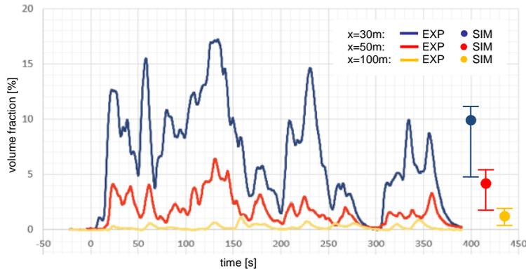
Figure 5: Comparison of maximum hydrogen concentrations during Test 4 (EXP) [6] compared with simulations from EFFECTS v12 (SIM)
