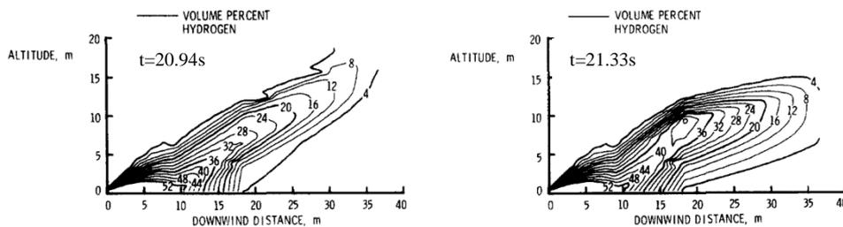
Figure 4: Temperature deduced hydrogen concentrations at  $t=20.94s$  (left) and  $21.33s$  (right) for NASA Test 6 (taken from [4])
