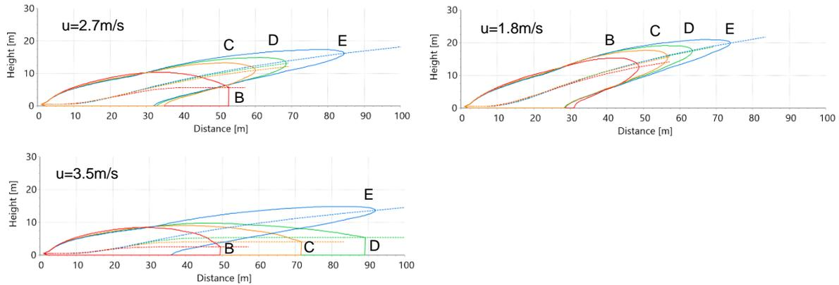
Figure 9: Simulations Test 6 (surface roughness length 0.1m) for different atmospheric stabilities and wind speed of 2.7m/s (a), 1.8m/s (b) and 3.5m/s (c); comparison of cloud dispersion behaviour shown by trajectory and plume contour (2% concentration v/v)
