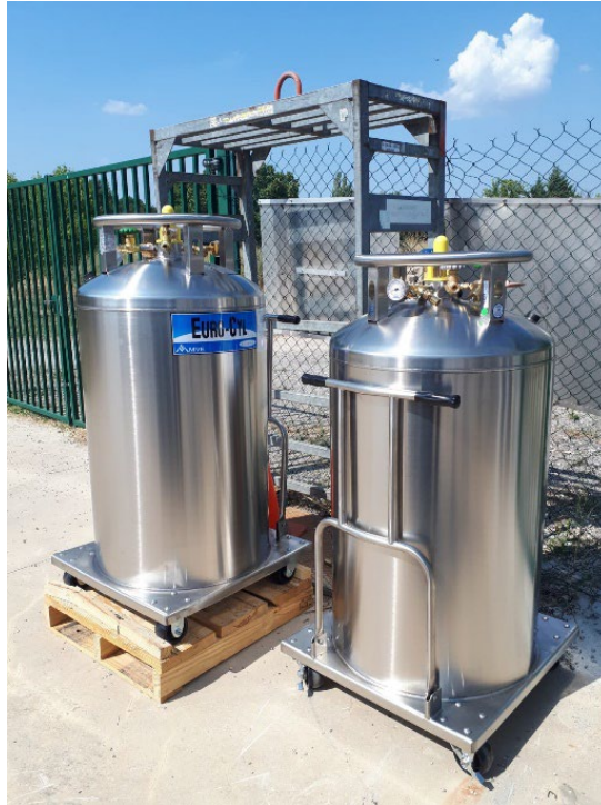
Figure 2. The two LIN tanks simulating a liquid hydrogen leak and dispersion in atmosphere.
