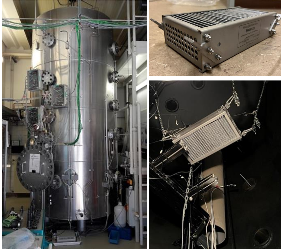
Figure 4. REKO-4 test vessel (left), EnerSys Hawker Hydrogen Eliminator (right, top), Recombiner installed inside the test vessel (right, bottom)
