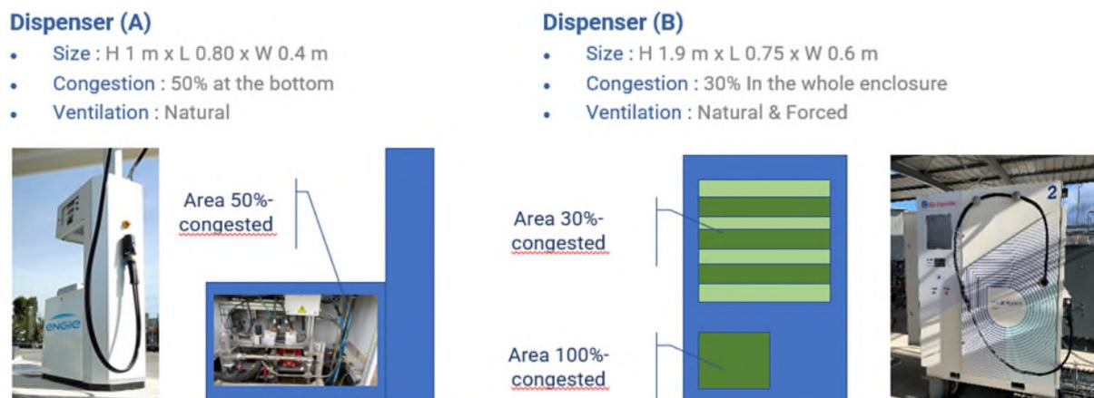
Figure 1. Geometries of the hydrogen dispensers studied
