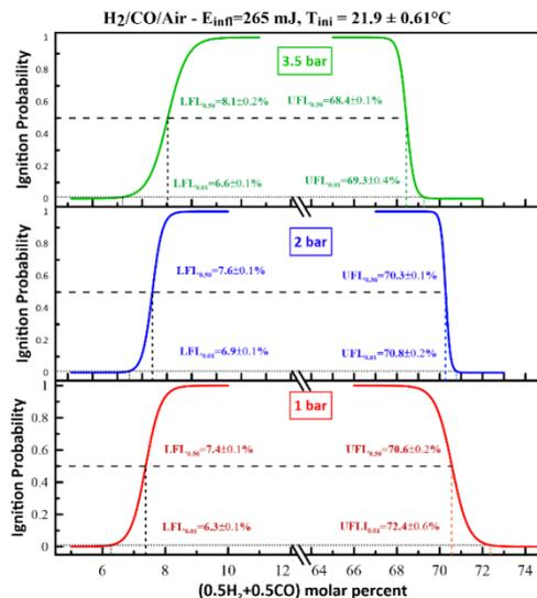
Figure 4. Probability of ignition versus the fuel/air molar percent. The binary fuel is constituted of
