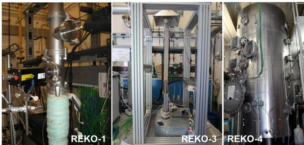
Figure 5. REKO facilities: Flow tube reactors for steady-state well-defined boundary conditions (REKO-1, REKO-3) and a pressure vessel for pressurized tests (REKO-4)
