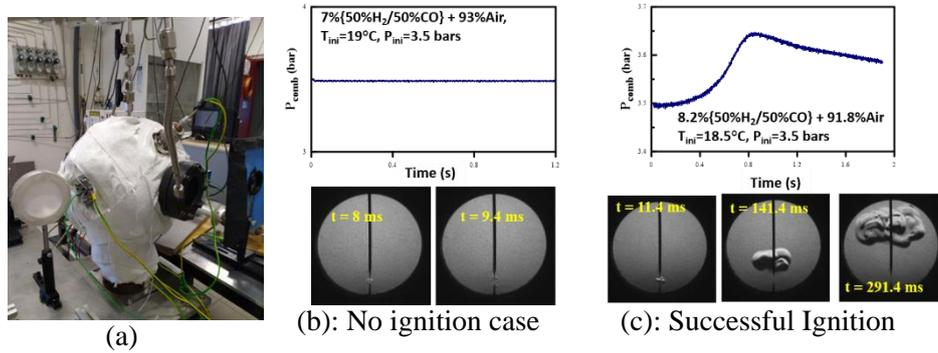
Figure 3. Experimental facility (BS-I) for the flammability limits study (a); examples of pressure signals and flame snapshots recorded for different runs in case of no ignition (b) and successful ignition (c).
