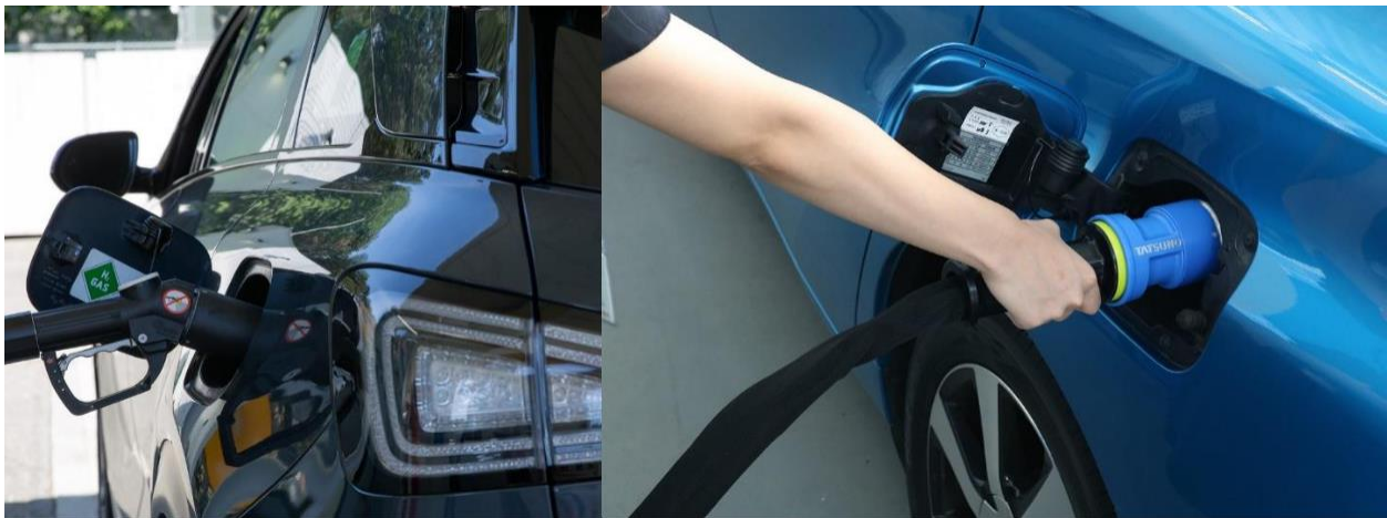
Figure 7. Left , A “pistol style” hydrogen nozzle connected to a Hyundai Nexu. Right , A “barrel style” hydrogen nozzle connected to a Toyota Mirai
