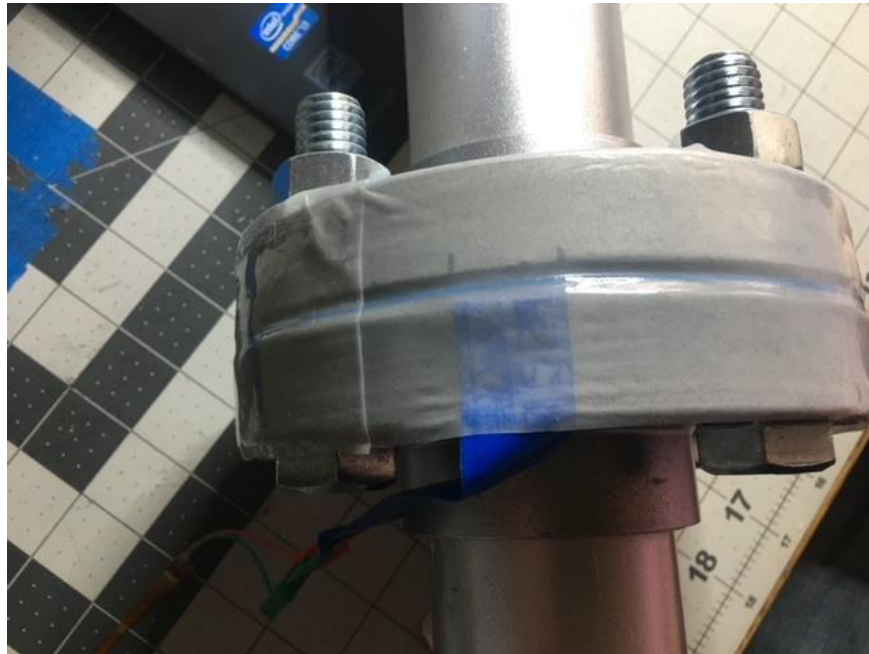
Figure 3. Mock flange assembly with an E1 resistive sensor wrapped in DetecTape®, remotely monitored with passive RFID and tested at a flow rate of 8 sccm
