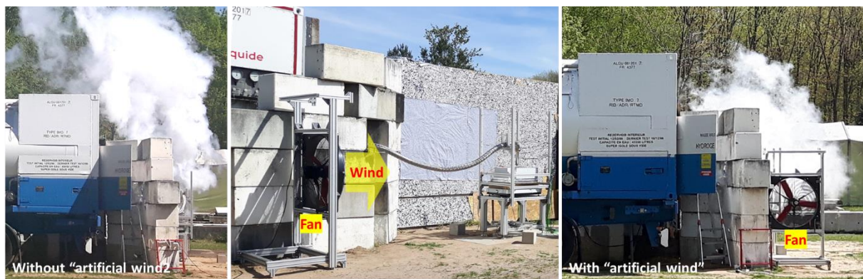
Figure 3. Photo of an experiment without “artificial wind” (left), experimental setup with fan (center) and experiment with “artificial wind” (right).
