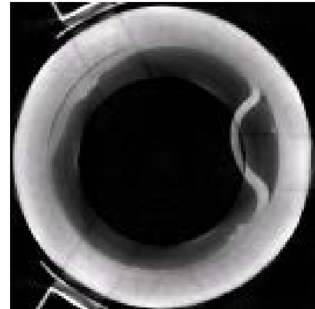
X-Ray tomography of a polymer liner pressure vessel
