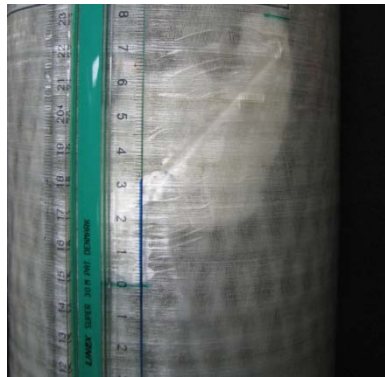
Impact visualisation on the glass fiber layer of a pressure vessel
