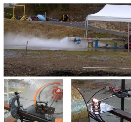
Figure: experimental set-up for ignition by hot surface
