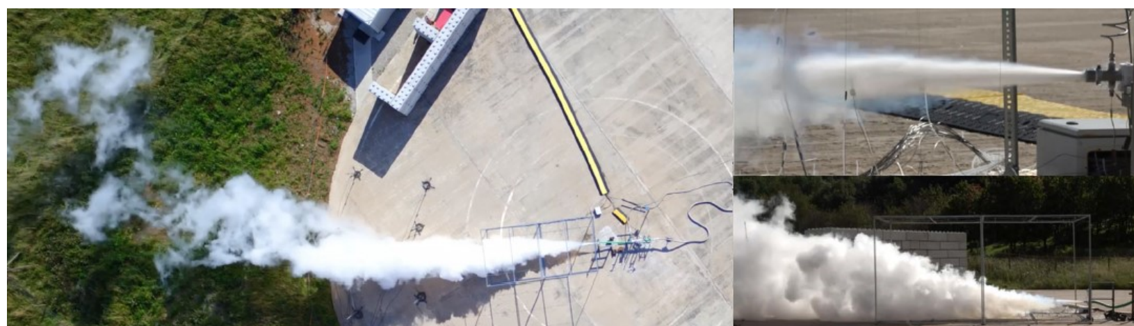
HSL experiments on dispersion and rainout of large scale LH2 releases
