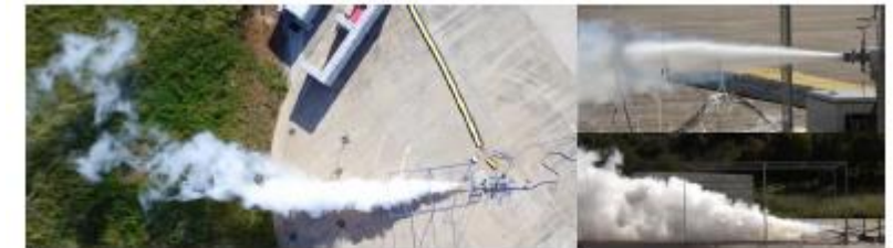
HSL experiments on dispersion and rainout of large scale LH2 releases
