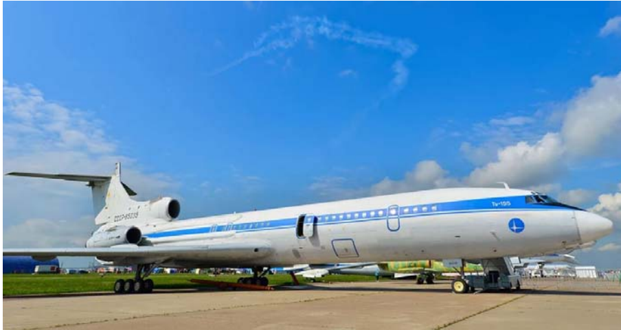
Figure 2-24. Tupolev 155 “Flying Laboratory” of 1988 with the central engine fueled by LH 2 or LNG (Courtesy of PSC Tupolev).
