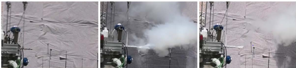
Figure 3-21. Optical observation from cold test with release diameter of 2 mm and pressure of 0.4 MPa.
