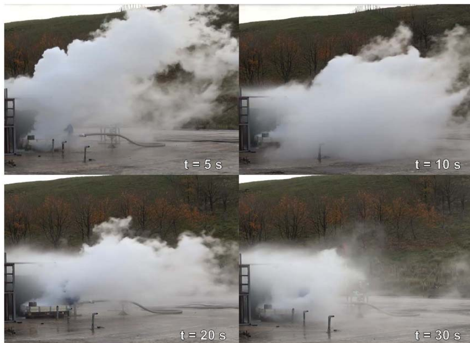
Figure 3-40. Vapor production after 5, 10, 20 and 30 s of water spray impingement.
