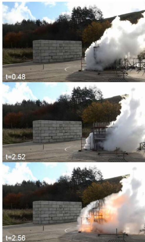
Figure 3-59. Pictures showing sudden gust immediately prior to ignition for test with release P=1\text{ barg} , d=12\text{ mm} , and wind velocity= 2\text{ m/s} .
