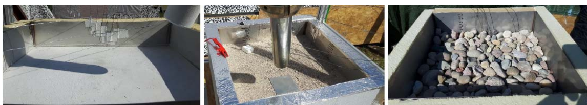
Figure 3-9. Experimental set-up for LH 2 pool investigation on different substrates: concrete, sand and gravel.
