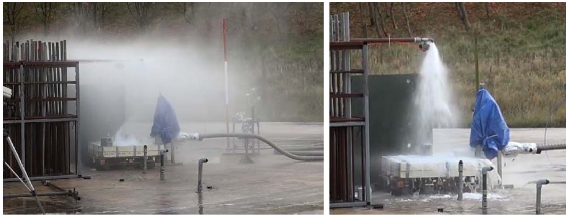
Figure 3-39. Experimental facility for rapid phase transition investigation.
