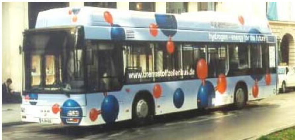
Figure 2-17. MAN hydrogen-driven fuel cell bus of 1996 with LH 2 storage tanks.
