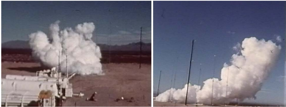
Figure 3-14. Cold hydrogen vapor cloud dispersion during NASA spill test #6. (Courtesy of NASA).
