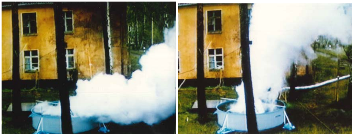
Figure 3-16. Screenshots from the evolving vapor cloud following LH 2 spill.
