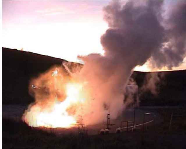
Figure 3-53. Ignition of the LH 2 vapor cloud during low wind conditions (no secondary explosion).
