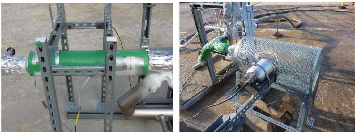
Figure 3-37. Experimental setup. Left: isolated pipework. Right: Faraday cage and field meter.
