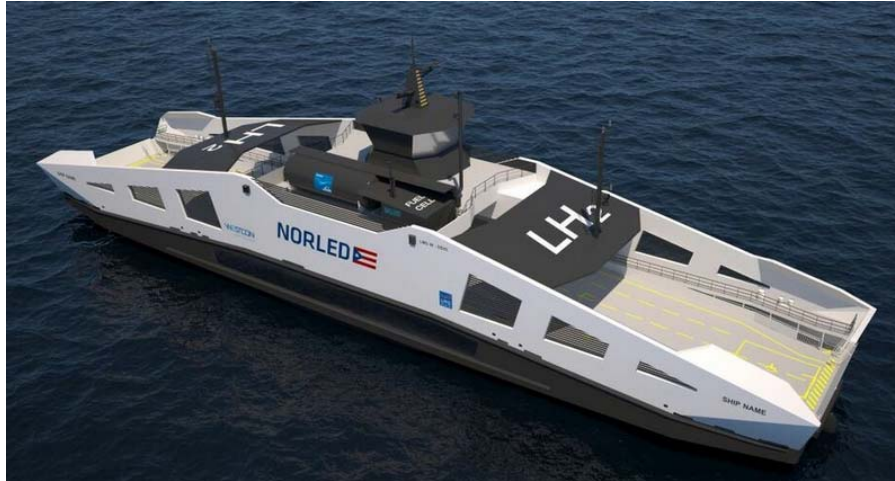
Figure 2-21. On-deck arrangement of LH 2 storage, fuel cell and vent mast on the NORLED ferry [NORLED 2019].
