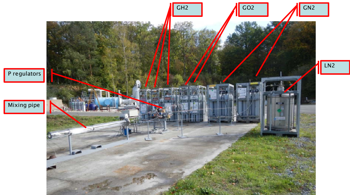
Figure 3-27. Details of the setup for T_{crit} measurements.
