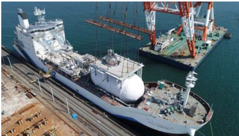
Figure 2-12. SUIISO FRONTIER, the world's first LH 2 carrier ship launched in 2019 with LH 2 storage tank [KHI 2020a].
