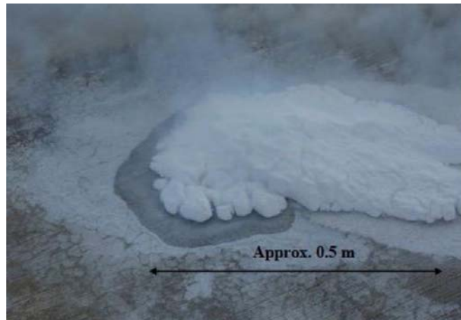
Figure 3-8. Solidified air formed during the LH 2 spill experiments.
