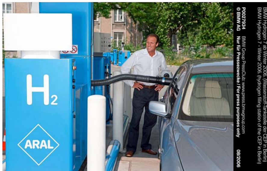
Figure 2-16. Refueling station for both GH 2 and LH 2 in Berlin (Courtesy BMW Group).
