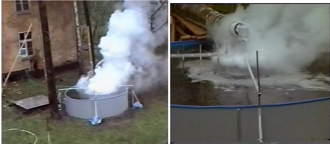
Figure 3-5. LH 2 pool spreading on water during spill tests in 1996 with ice layer visible at test end (Courtesy of BAM).
