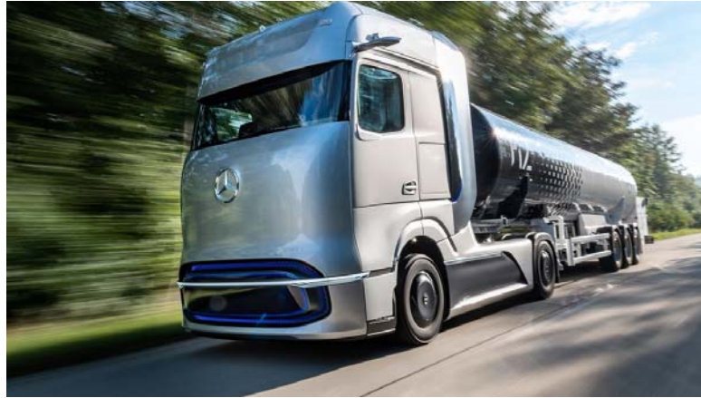
Figure 2-19. Mercedes FC truck GenH2 concept with LH 2 storage.
