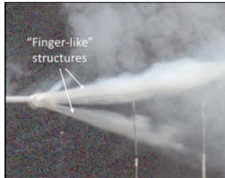
Figure 14: Photo of the “finger-like” structures that formed at the tip of the nozzle during this experiment (Friedrich, Vesper, & Jordan, 2020)
